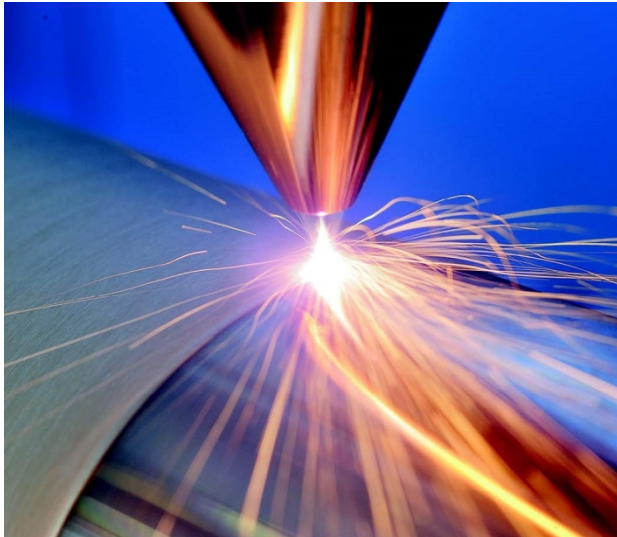
Image 7: Technologies for Additive Manufacturing such as the extreme High-Speed Laser Material Deposition (EHLA) were a hot topic at AKL'18. © Fraunhofer ILT, Aachen, Germany / Volker Lannert.
