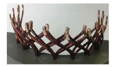
Laser cutting and welding for electro motors, e.g. hairpin
