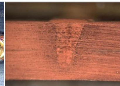
Penetration depth: 1,63mm P_{av} = 5,7 kW
