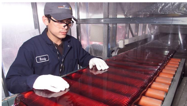
Image 3: A production line was set up on site during the construction of the National Ignition Facility (NIF) specifically for the manufacture of the laser glass plates. © Lawrence Livermore National Laboratory.
