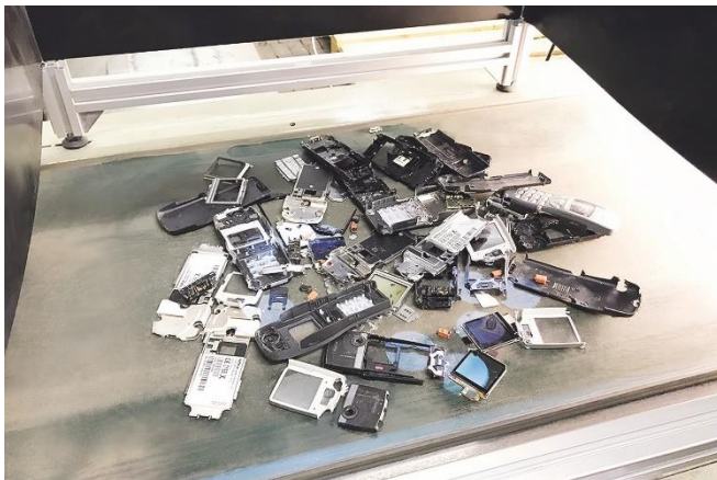
Image 3: Successful recycling in the ADIR project led by Fraunhofer ILT: by disassembling around 1000 mobile phones and over 800 printed circuit boards, the researchers sorted several kilograms of components for recovery of valuable metals.
