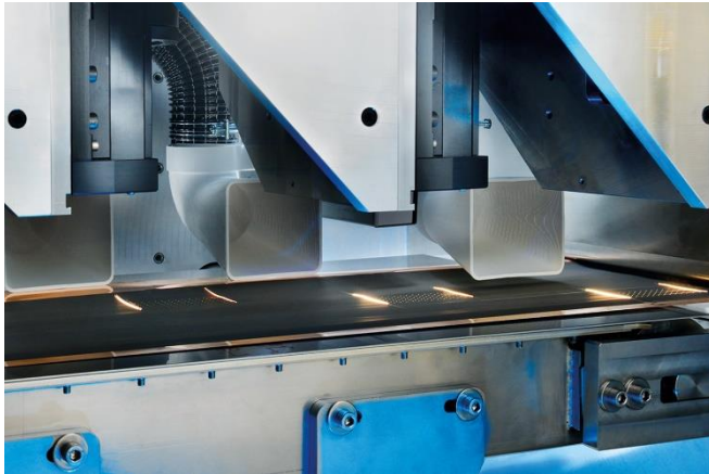
Image 2: High throughput: When creating the hole structures, the ultrashort pulse laser works with four scanner modules, each equipped with six beamlets. © Fraunhofer ILT, Aachen, Germany.
