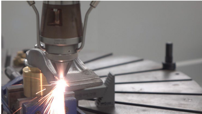
Image 1: Coating of excavator teeth using Laser Material Deposition (LMD). ©Fraunhofer ILT, Aachen, Germany.
