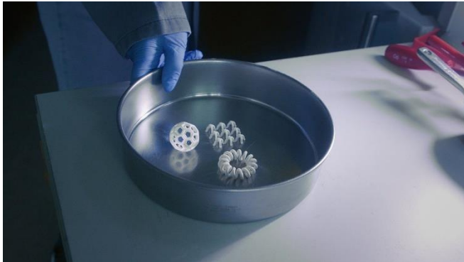
Image 5: SLS polymer parts: filigree lattices and functional samples for design, material, and process testing. Fraunhofer ILT's flexible lab systems support small powder batches and rapid material changeovers. The focus is on new materials such as very soft TPU and shape memory polymers. © Fraunhofer ILT, Aachen, Germany.
