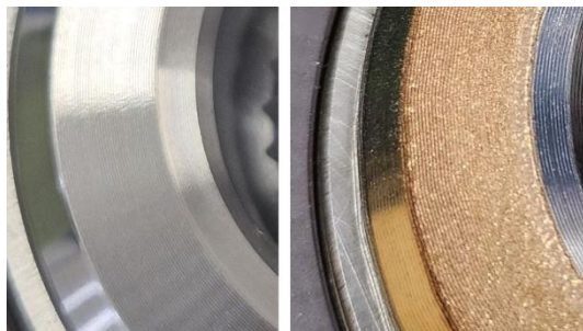
Image 5: Not all roughness is a disadvantage: The investigations showed that the structure of the EHLA layer can absorb protective and lubricating substances, thereby contributing to a stable contact surface. © LJIN GmbH.
