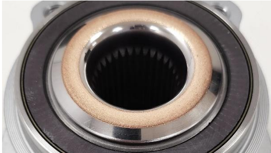
Image 1: The fully coated Generation 3 wheel bearing unit from ILJIN: The EHLA functional layer is applied to the ring surface where the interface with the drive shaft is formed in the vehicle. It specifically modifies the contact surface without introducing an additional component into the confined installation space. © ILJIN GmbH.
