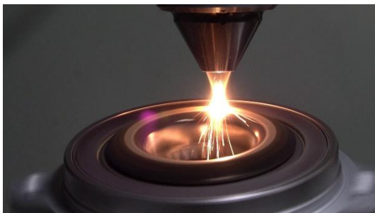
Image 2: In extreme high-speed laser material deposition (EHLA), metal powder is melted by the laser beam and applied to the component as a thin functional layer. For the wheel bearing application, it was crucial that the coating process be cost-effective and efficient, and introduce minimal heat into the base material. © Fraunhofer ILT, Aachen, Germany.
