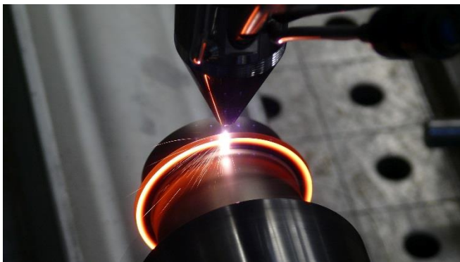
Picture 2: Ultra-high-speed laser material deposition (EHLA): protection against wear and corrosion, repair and additive manufacturing - all with only one system technology. © Fraunhofer ILT, Aachen, Germany.
