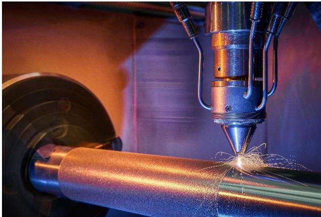
Picture 1: With EHLA, metal protective layers can be applied with ultra-high-speed. © Fraunhofer ILT, Aachen, Germany / Volker Lannert.
