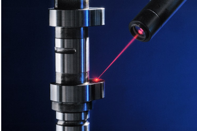
Picture 1: INSPIRE-Sensors for testing shape and positional tolerances on camshafts. © Fraunhofer ILT, Aachen, Germany.
