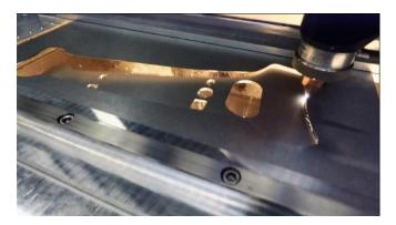
Image 2: Instead of punching: Together with BILSTEIN GmbH & Co. KG, Fraunhofer ILT has developed a very fast cutting process for differentiated rolled strip with partially different properties. © Fraunhofer ILT, Aachen, Germany. PRESS RELEASE August 30, 2018 || Page 4 | 4
