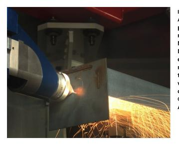
Image 1: A multifunctional laser processing head plays a major role in the new NRW project MultiPROmobil; it enables innovative sheet metal assemblies through the integrated cutting, welding and manufacture of structures additively. © Fraunhofer ILT, Aachen, Germany. PRESS RELEASE August 30, 2018 || Page 3 | 4
