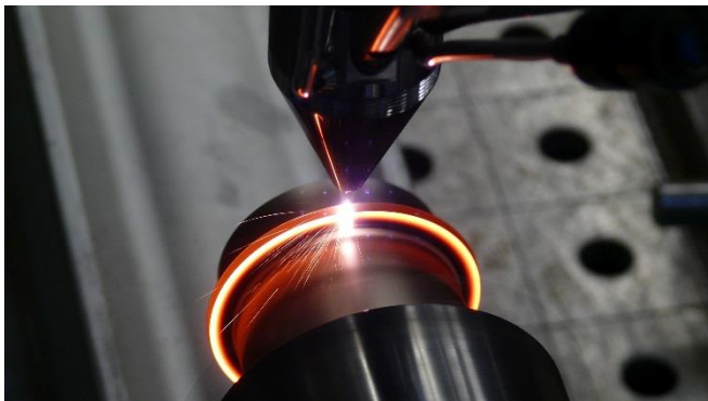
Image 2: Extreme high-speed Laser Material Deposition (EHLA): protection against wear and corrosion, repair and additive manufacturing – all with only one system technology. © Fraunhofer ILT, Aachen, Germany.
