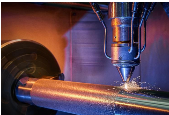
Image 1: Demonstration: A video at the ILA Berlin Air Show shows how quickly, precisely and efficiently EHLA Laser Material Deposition works. © Fraunhofer ILT, Aachen, Germany / Volker Lannert.
