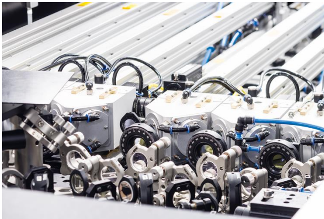
Image 2: Coherently combined USP fiber lasers of the kW class, as they are made available in the user facility at Fraunhofer IOF. © Fraunhofer IOF, Jena, Germany.
