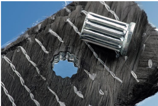
Image 3: USP laser beam drilled carbon-fiber preform with a star-shaped hole and positive-fit metal insert. © Fraunhofer ILT, Aachen, Germany.
