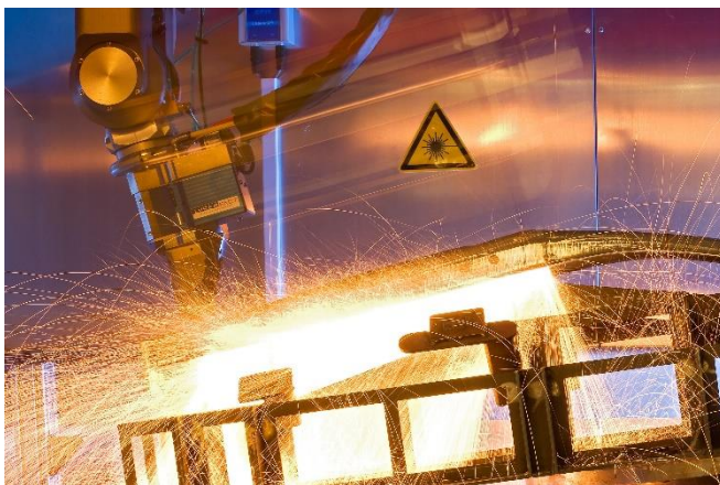
Image 2: Processing of an automotive structural component with the multifunctional laser tool. © Fraunhofer/Thomas Ernsting.
