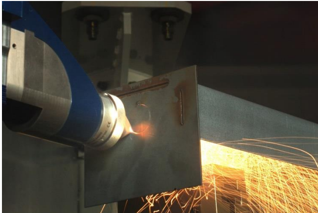
Image 1: Multifunctional laser processing head that can already cut and weld innovative sheet metal assemblies. Now, additional additive manufacturing steps are added. © Fraunhofer ILT, Aachen.
