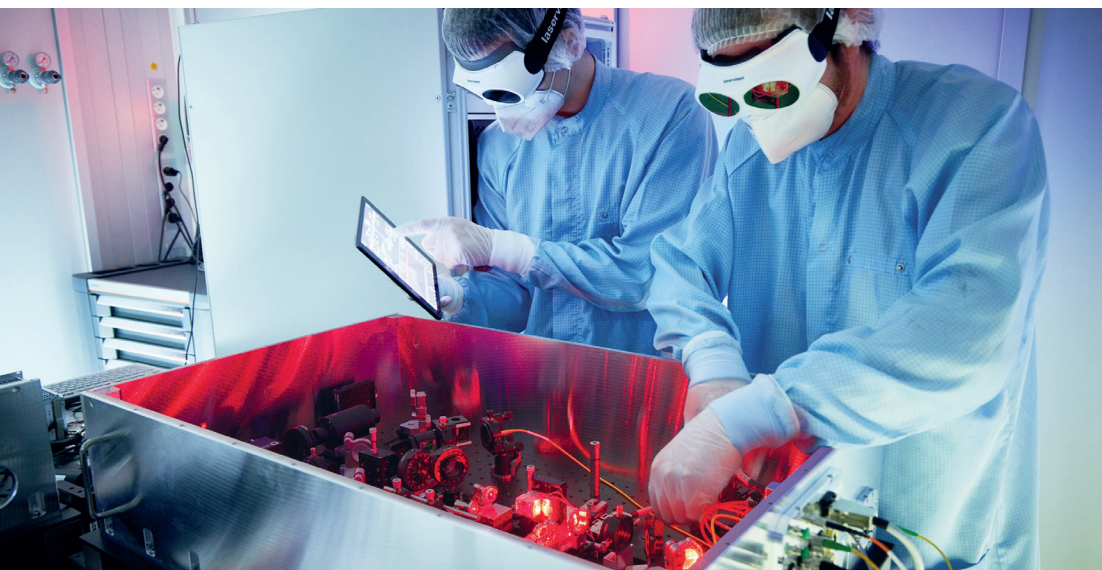
Adjustment of the converter using an attenuated red laser to emulate the single photons.
