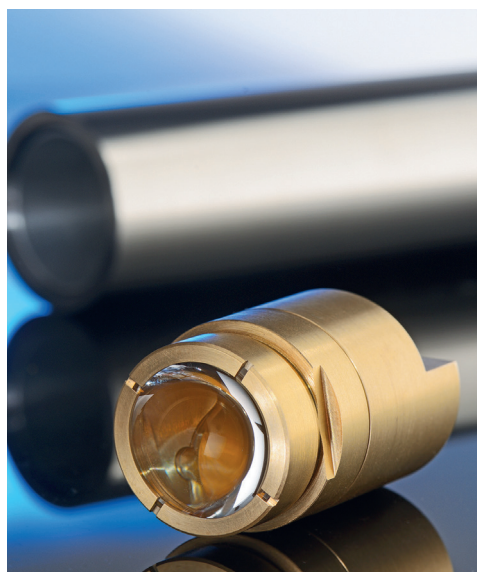
1 Aachen-Soers wastewater treatment plant of the Eifel-Rur Water Board (WVER). 2 Immersion probe for 2D fluorescence spectroscopy.
