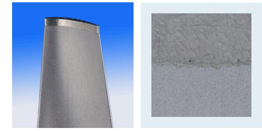
1 Transition between LPBF area (top) and cast base component. 2 Microstructure of the bonding zone between the base material and the LPBF area.
