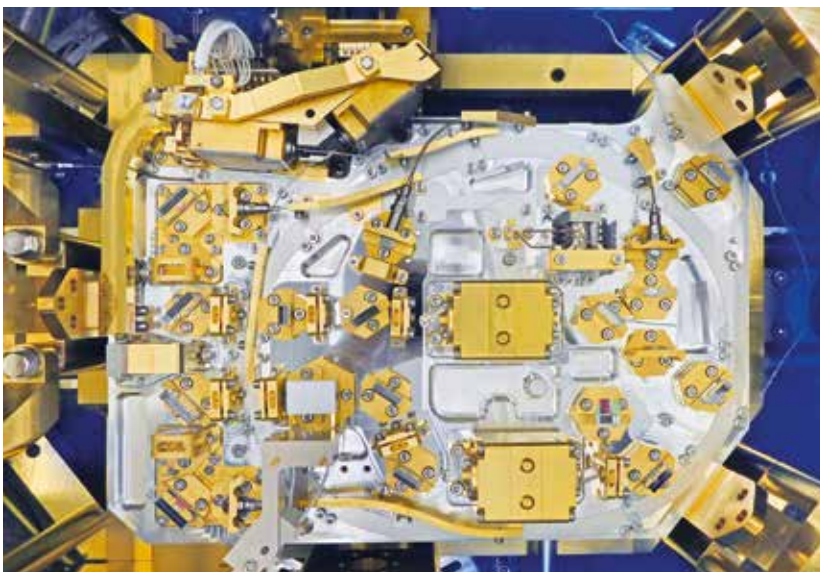
Finished oscillator of the EQM.
