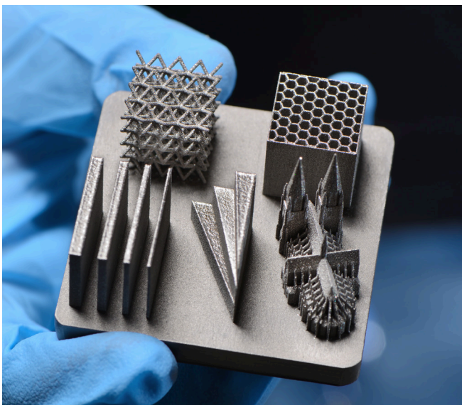
Demonstrator components for adaptive LPBF process control.
