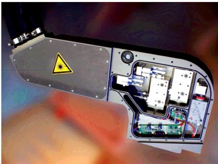
Optical system with focus position control and monitoring
