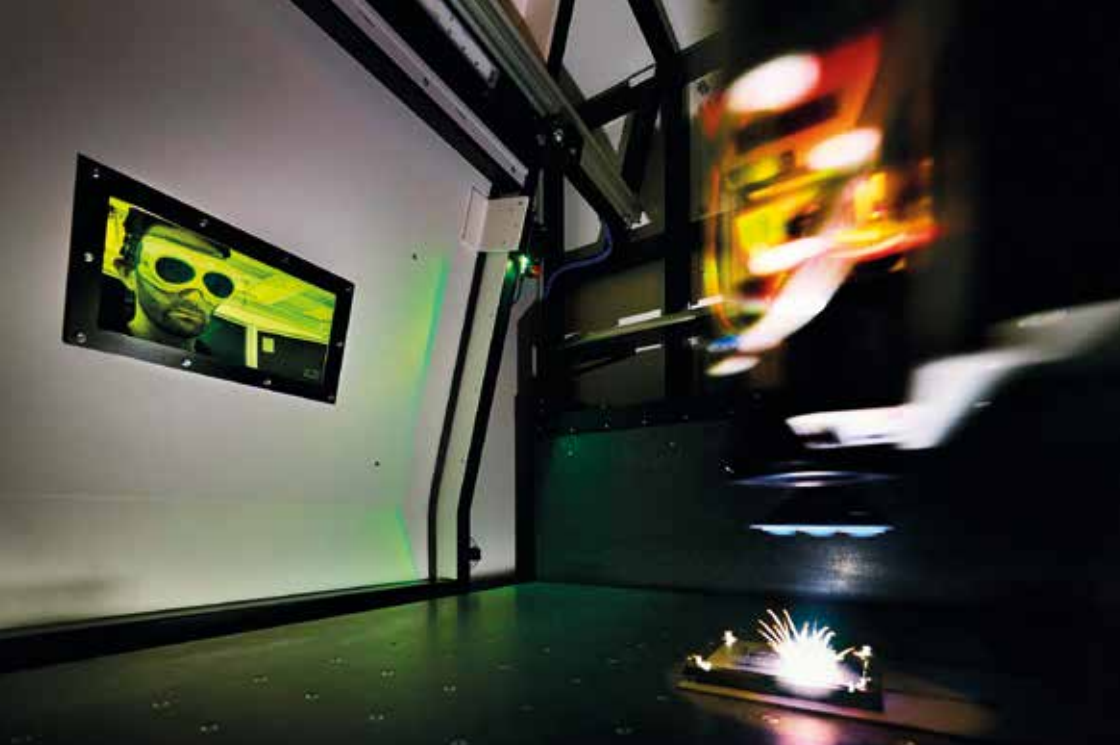
Laser processing of bipolar plates for fuel cell production at Fraunhofer ILT.
