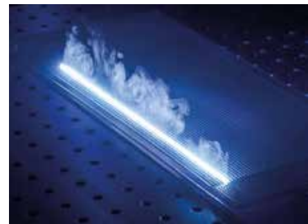
Large-area coating removal of a compound bipolar plate.
